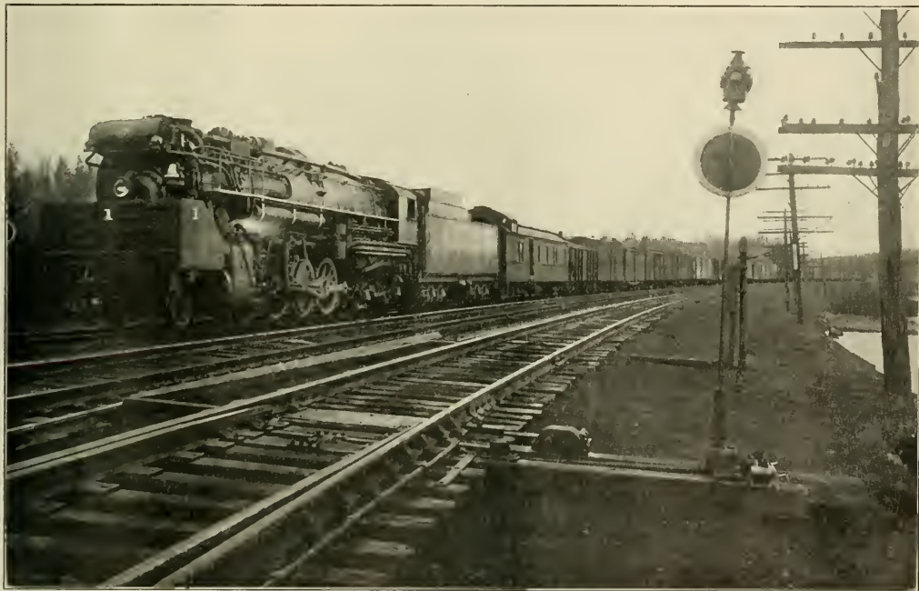
Lima Locomotive Works 2-8-4 Type Locomotive With Test Train on the Boston & Albany Railroad
